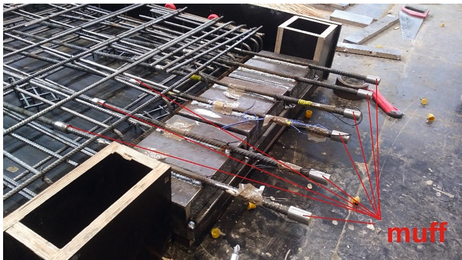
Fig. 4. Balcony connection with glued strain gauges before concreting set II_ZB_2_3 – muff on longitudinal reinforcement bars (Stage II) [own study]
