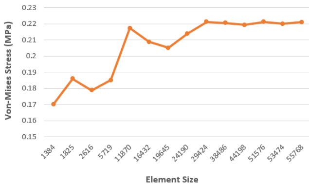
Fig. 7. Maximum Von Mises stress vs. mesh element size.
