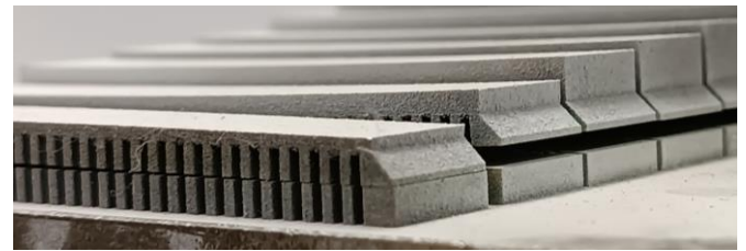
Fig. 7. Photograph of the specimen with 1 mm bar thickness
