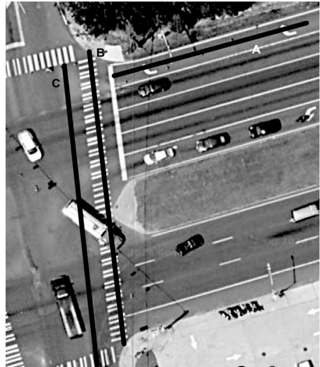
Figure 1. Suburban intersection (Google Maps). Measurement lines: line A - drivers approach, 100 feet; line B – pedestrian intended path, 146 feet; line C intersection with vehicles approaching from the drivers' right, 157 feet.
