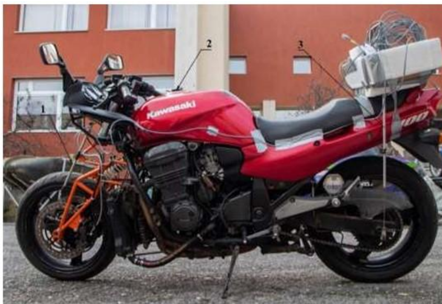
Figure 1. Kawasaki GPZ 1100 equipped with sensors and computer
