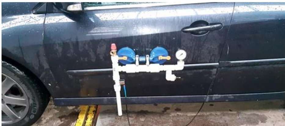
Figure 8. A prototype of the Brake-Marker device mounted on a vehicle
