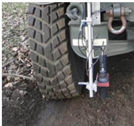
Figure 2. Datron sensor mounted in a military vehicle
