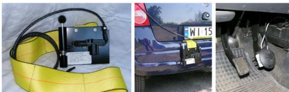
Figure 3. "Shot marker" device installed in an Opel Agila vehicle. Source: (Drobiszewski et al. , 2015)
