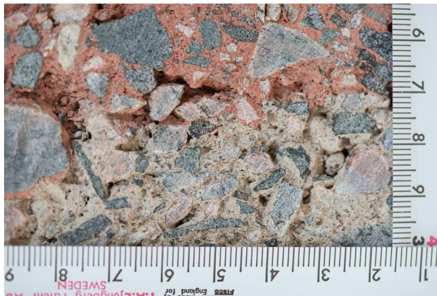
Figure 2. Internal pore structures arising in connection with manufacturing. Photo: Per Lindh
