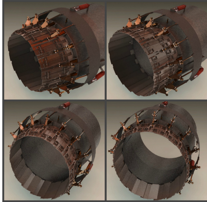
Fig. 7. Subsonic nozzle with TVC in different positions.
