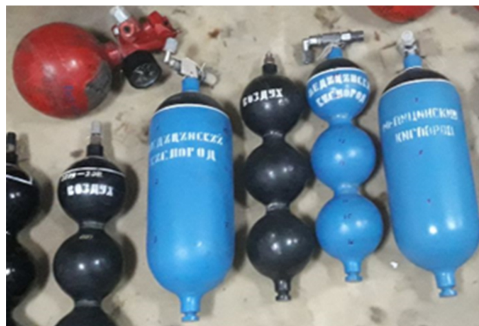
Fig. 7. Spherical and cylindrical gas containers of aircraft selected for NDT inspection
