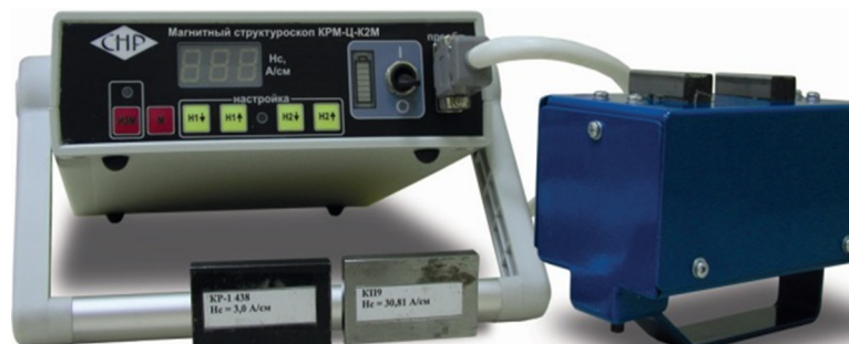
Fig. 5. The KRM-Ts coercive force meter with attachable U-shaped core magnetic transducer and two calibration specimens of known coercive force
