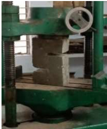
Fig. 2 Testing push-off specimen
