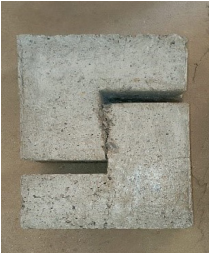
Fig. 3 Failure mode of specimen
