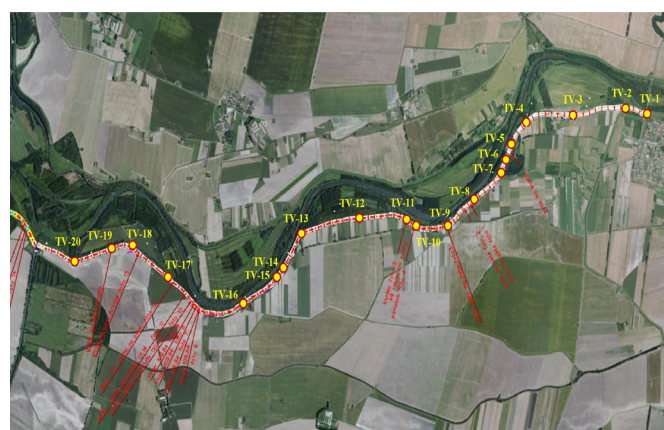
Fig. 2 Layout of exploratory boreholes TV-1 to TV-20 on the right-hand side of the levee of the Little Danube between the Kolárovo and Aszód pumping stations, which shows the occurrence of surface leaks during the flood flows in 2006
