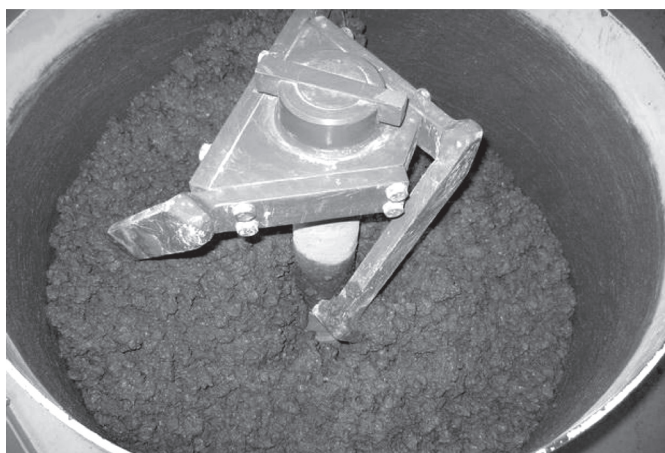
Fig. 3 Horizontal mixing of a concrete batch
