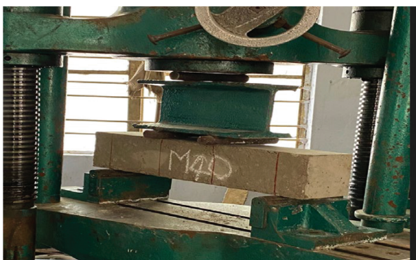
Fig. 7. Testing of GPC beams with UTM
