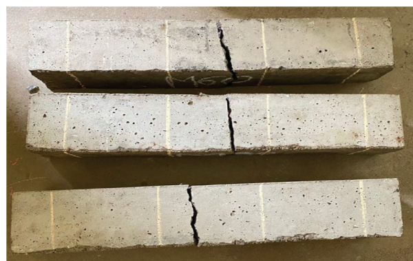
Fig. 8. GPC beams after testing
