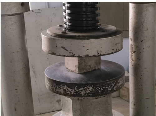
Fig. 2. Testing of a GPC cube with CTM
