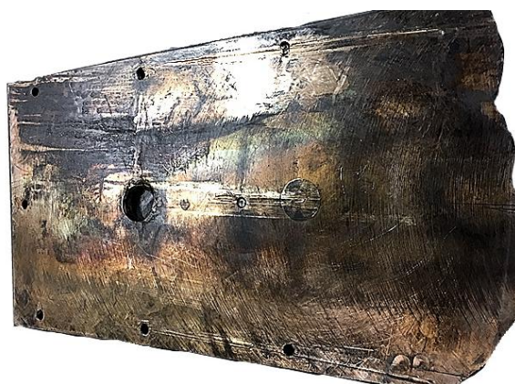
Fig. 9. Damaged (broken) slide plate of the ram guide
