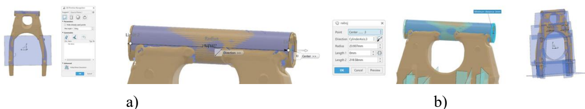
Fig. 2 CAD reconstruction of the swingarm in Dassault Systèmes 3DEXPERIENCE; (a) surface reconstruction of scanned geometry, (b) solid model with functional features (bearing housings, wheel mounts) prepared for further optimization
