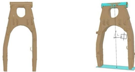
Fig. 1 Initial CAD model of the motorcycle swingarm obtained by 3D scanning and reconstruction
