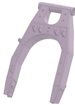
Fig. 4 CAD reconstruction of the swingarm in 3DEXPERIENCE; (a) surface reconstruction, (b) solid model
