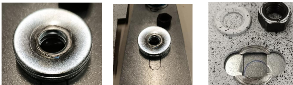
Fig. 16 Due to the large bending deformation of the washer 1 (on the left side), the actual contact surface is smaller and therefore the contact pressure will be much higher; due to the very small contact area of the washer 2 , (on the right side) the contact pressure is also too high
