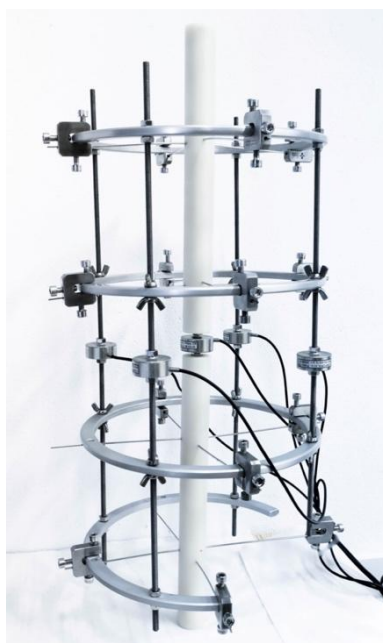
Fig. 1 Model of external fixator with measuring sensors
