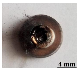
Fig. 8 Low-quality element with blowhole unmasked after joining using the RES
