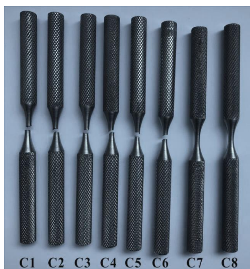
Fig 6. Condition of 8 specimens as-cast Ti-6Al-4V after undergoing the dynamic fatigue test.
