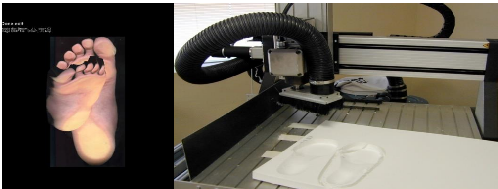
Fig. 2 Left – insole design based on the digitization results of the plantar foot surface; Right – three-axis CNC milling machine typically used for manufacturing the base of orthopedic insoles.
