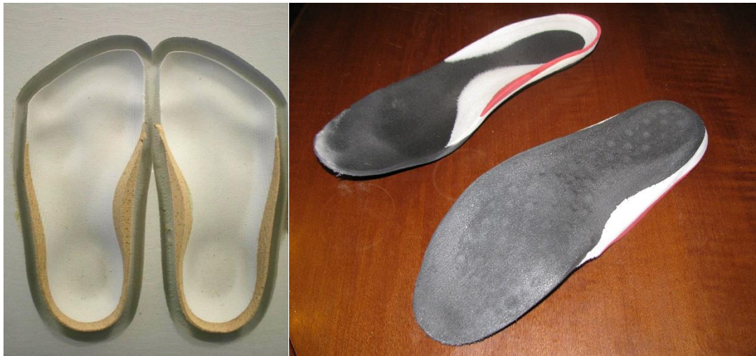
Fig. 8 Insoles made using the IPASIOU system. Left - pair of newly made insoles; Right - pair of insoles after 5 years of use.
