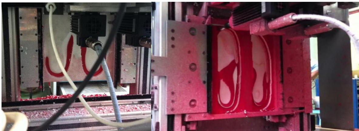
Fig. 7 Processing of EVA material block for making orthopaedic insoles. Left: processing the lower sides of the insoles; Right: processing the upper surfaces of the insoles.
