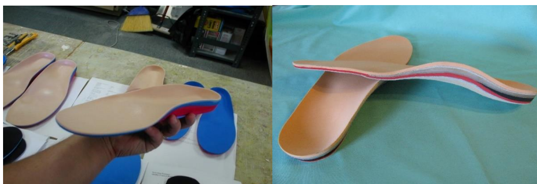
Fig. 1 Custom-made orthopedic insoles using CAD/CAM technology. Left: base of the insole made by direct processing of EVA material; Right: base of the insole made by thermoforming on a produced mold.
