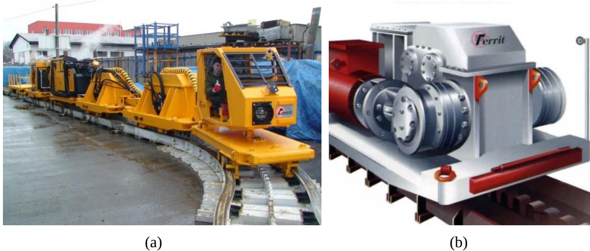
Fig. 1 Rack-railway track (a) Whole system, see [6], (b) Detail – an example of a train unit
