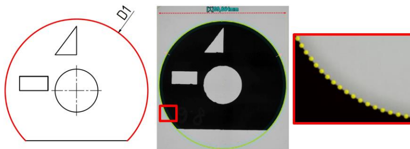
Fig. 4 Graphic representation of the response measurement on the outer circle D1.
