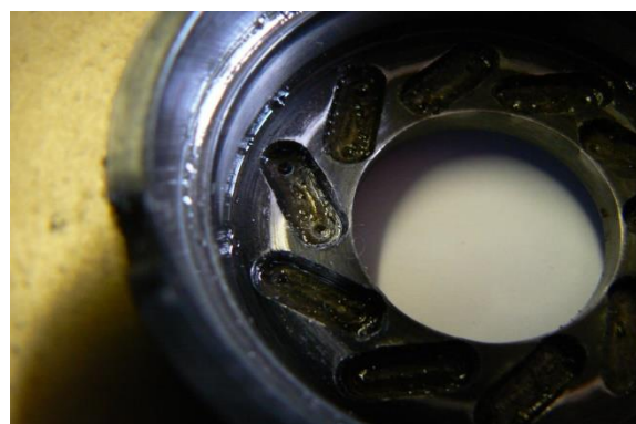
Fig. 8. Overrunning ball clutches of the rear hub of the bicycle: a - cross-section of the overall view of the clutch; b - view from the end face of the driving semi-clutch; c - view from the end face of the driven semi-clutch.
