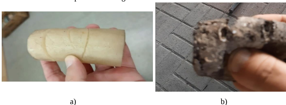
Fig. 9 Transverse cracks in the pigs after they pass through the tees: a) – a pig made of an elastic polymer composition; b) – a pig made of silicone sealant
