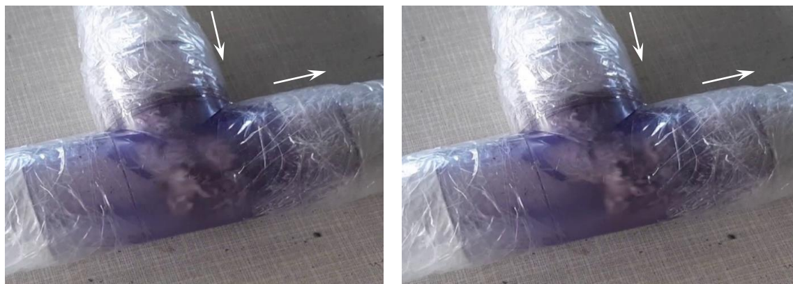
Fig. 13 The movement of the pig through the tee, in which the flow and the pig enter the branch of the tee, and exit to one of the sides of its trunk (the modulus of elasticity for bending of the material from which the pig is made is small)
