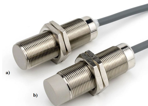
Figure 1. Examples of inductive proximity sensors shielded (a) and unshielded (b) [11].
