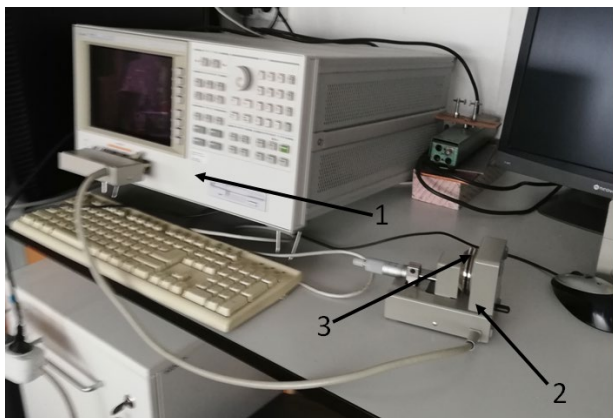
Figure 4. Experimental configuration of the dielectric measurement: Agilent 4294A impedance analyzer (1), measuring cell 16451B (2), sample (3).
