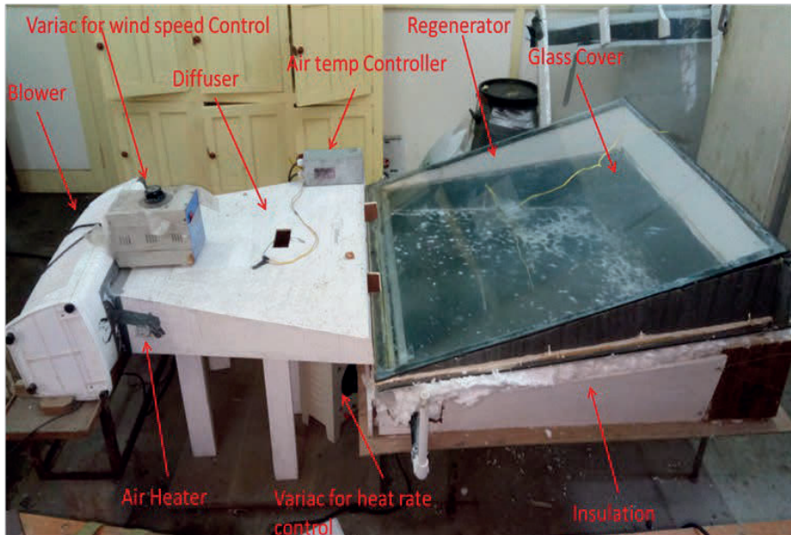
Fig. 1. Experimental set up for indoor regenerator testing with heat and wind generation facility.
