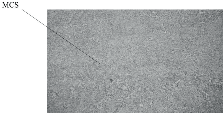
Fig. 2. Microcrystalline structure (MCS) observed within the massive, solidified layer, typically obtained under conditions of low cooling rate, maximum roller gap H = 10 mm.
