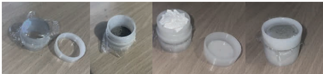
Fig. 2. XRF sample cup preparation.
