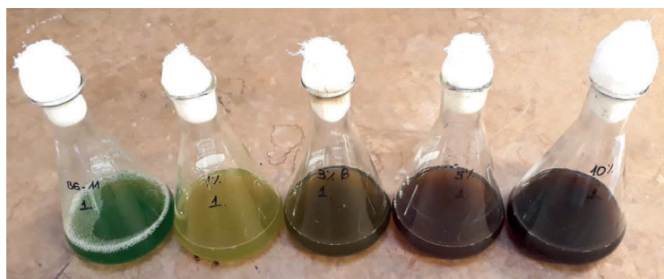
Fig. 3. C. vulgaris cultivation in various dilutions of digestate. Flasks from the left to right: control, 1 %, 3 %, 5 %, and 10 % digestate as a growth medium.
