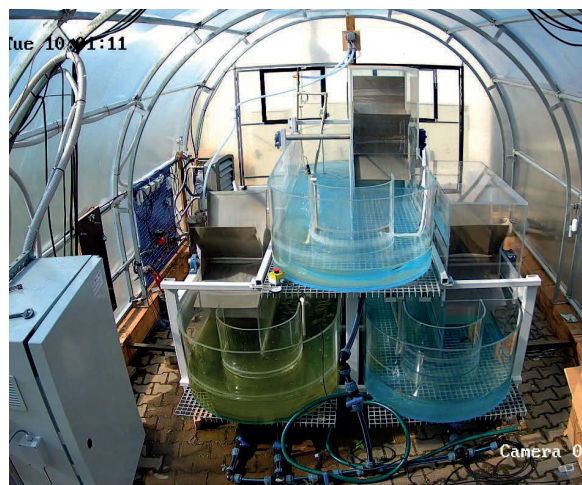
Fig. 1. Novel microalgae biomass production unit integrated into a biogas plant.
