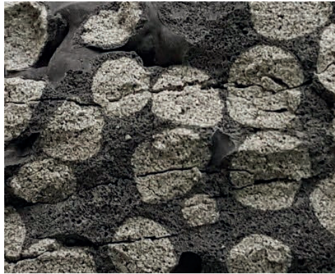
Fig. 4. Nature of concrete destruction during strength testing.
