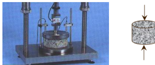
Figure 3. Triaxial cyclic compression test
