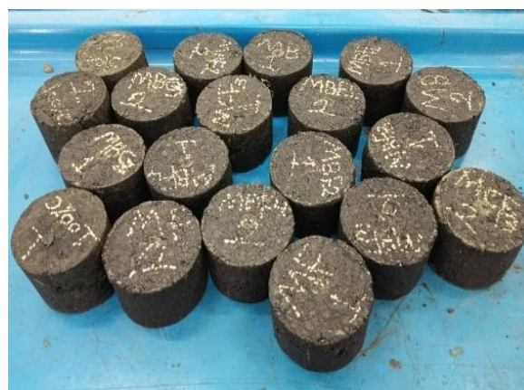
Figure 8. Asphalt concrete samples for MS testing.
