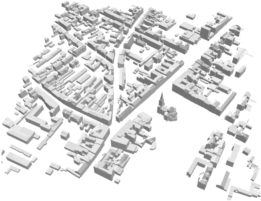
Fig. 7. Building models in CityGML 2.0 standard (LoD2) used in the analysis. Source: own elaboration.
