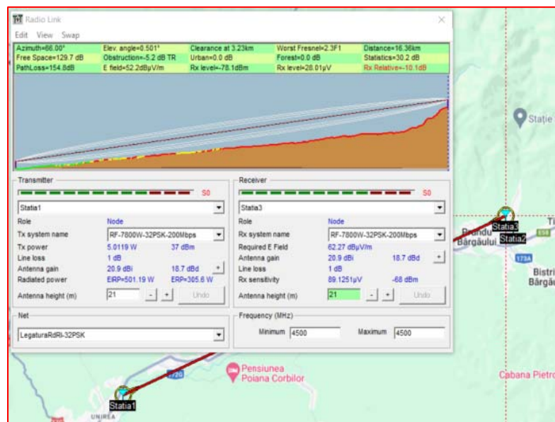
Figure no. 5: Result of the radio-relay link for 32PSK modulation
