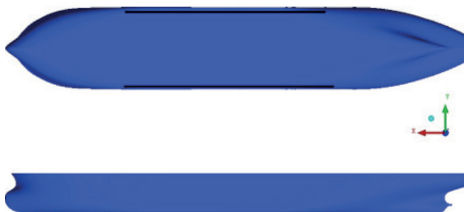
Fig. 11. Parallel side strakes added below and on the edges of the parallel part
