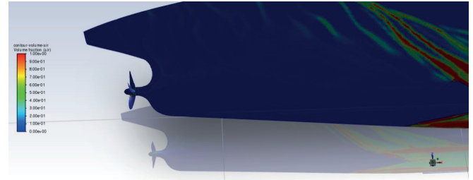
Fig. 27. Air leakage before reaching the propeller
