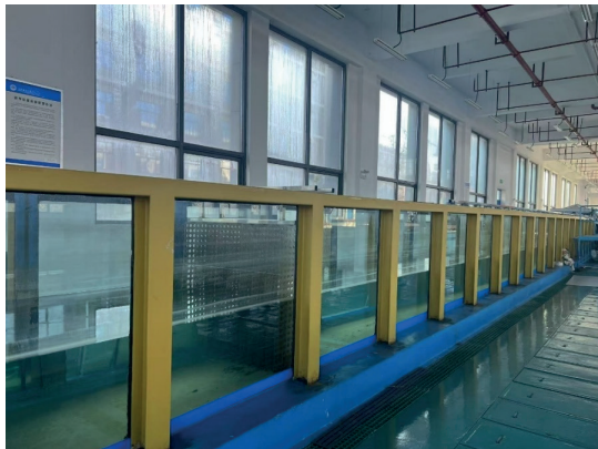
Fig. 3. Experimental flume for wind and wave currents at Jiangsu Ocean University
