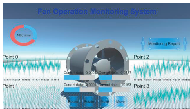
Fig. 13 Operation monitoring of the fan at 1000 r/min
