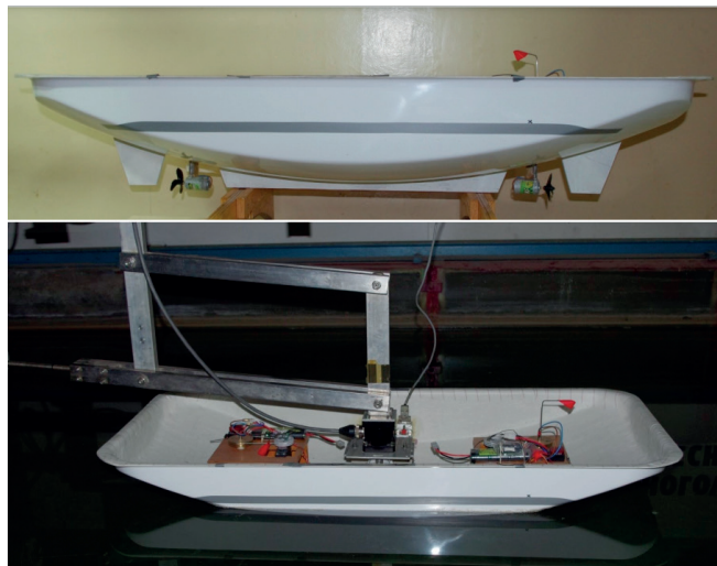
Fig. 2. Model with protruding parts (top), and during the tests (bottom)
