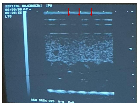
Figure 4. GE Healthcare LOGIQ α 100, linear transducer. A partially homogeneous area with grainy noise; artifacts in the form of black spots.
