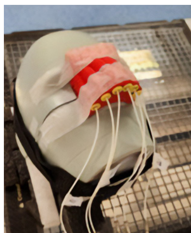
Figure 3. Head of the CIRS anthropomorphic phantom with a 3D bolus mounted on it.
