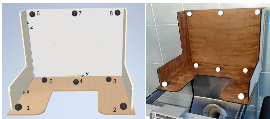
Figure 2. Calibration frame with eight visible markers. Their numbering defines the order of assigning coordinates. The assumed real-world coordinate system is marked by the axes on the CAD design visualisation (left). The real frame with markers shown on the phantom tank (right).
