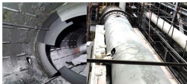
Figure 1. Diagram of the fracture location of the revolving tube
