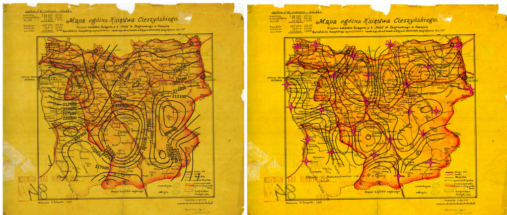
Fig. 6. Scale variation isolines with an interval of 2000 generated in Surfer (left) and isolines of scale variation with an interval of 5000 constructed in MapAnalyst (right) (prepared by M. Kuźma)
