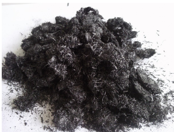
Figure 2. Biocarbon obtained during the torrefaction of flax shive (temperature - 250°C, process time - 10 min)
