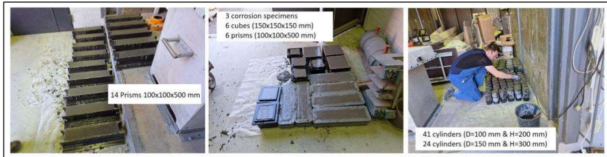
Figure 3 – Casting of the test specimens for each concrete mixture.
