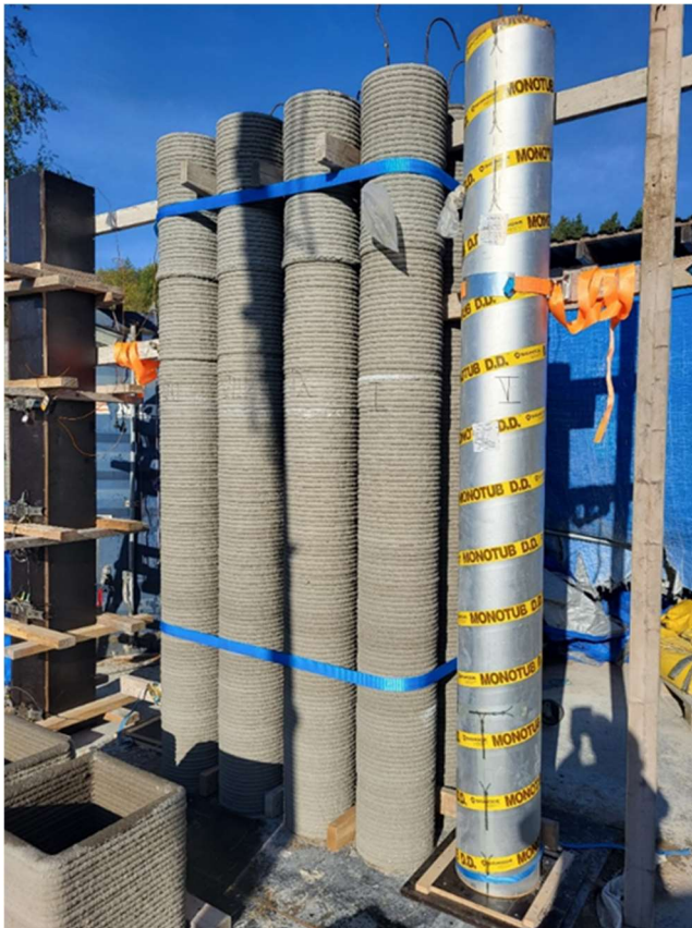
Figure 6 – 3DPC forms and cardboard form before casting the SCC. Please, note the wooden form to the very left of the photo. It was instrumented for measuring form pressure.
