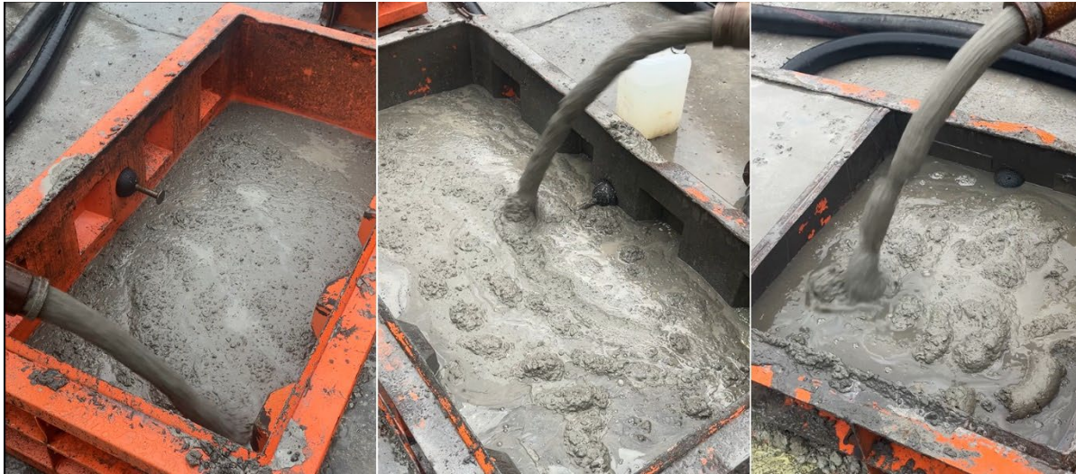
Figure 6 – Results from test 3. Left: 20 metres, 64 mm extension hoses, Middle: 40 metres, 64 mm extension hoses Right; 60 metres, 64 mm extension hoses.
