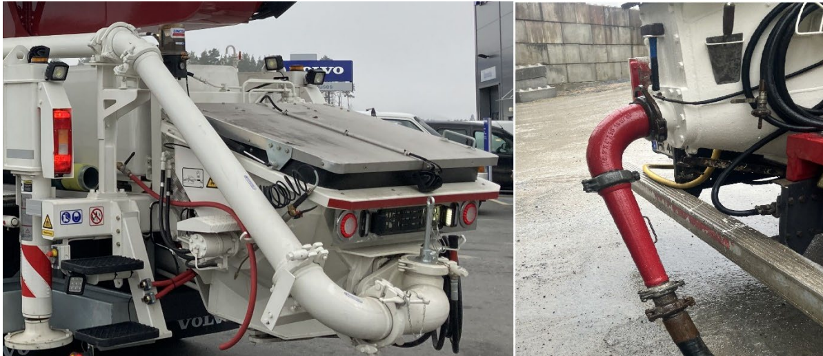
Figure 7 – Left: Concrete hopper outlet with U-bend and ball stopper, reducer, and boom. Right: Line pump concrete hopper outlet with bend and reducer.
