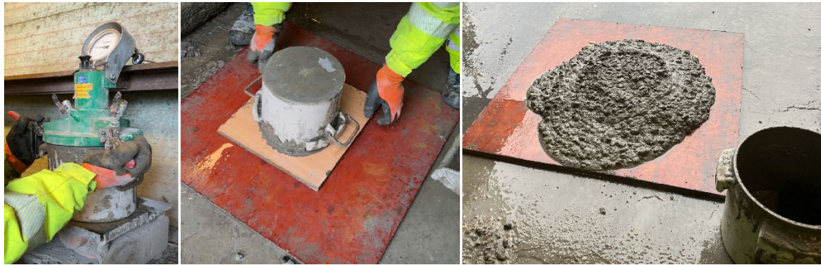
Figure 5 – Left: Applying pressure to fresh concrete using standardised apparatus for air content measurement. Middle: The bucket has been turned upside down utilising a plate to keep the concrete in the container. Right: Concrete ready to be measured, after bucket has been lifted.
