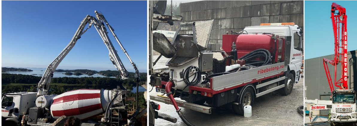
Figure 2 – Left: Pump mixer with 28 metres boom. Middle: line pump. Right: Boom pump with 43 metres boom.
