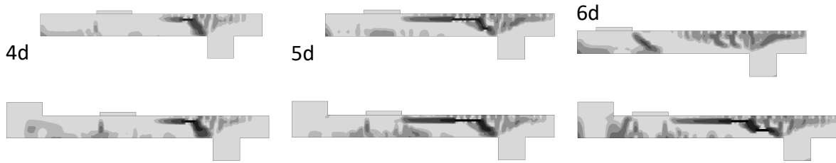
Figure 14 – Shear crack at the central transversal cross section of tests 4d, 5d and 6d with a b of 13 m.
