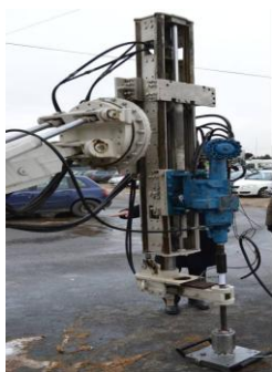
Fig. 7 Drilling feed frame positioned for testing
