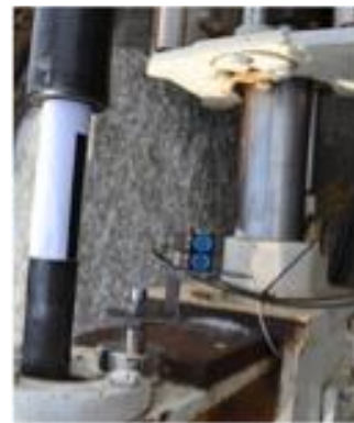
Fig. 4 Optical system for measuring the rotational speed of the rod
