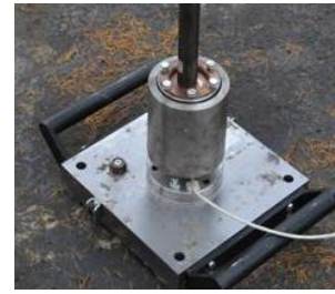
Fig. 3 View of the force sensor housing equipped with an elastomer insert
