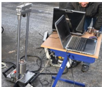
Fig. 6 Station with a built-in measuring and recording system for calibrating the force sensor
